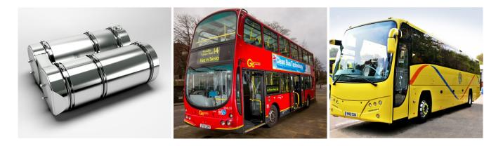
The Eminox SCRT<sup>®</sup> system can be retrofitted to heavy duty vehicles to achieve real world emissions, equivalent to Euro VI. Our latest SCRT<sup>®</sup> technology can deliver NOx and NO<sub>2</sub> reduction of 99%.
