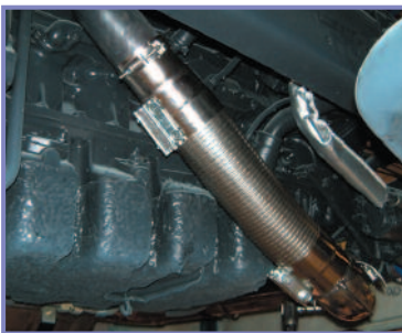
Figure 22 - Typical flexible pipe used to isolate vibration
