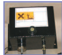
Figure 4 – metal additive tank
