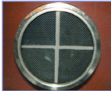
Figure 21 - Outlet face of a used filter
