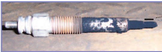
Figure 23 showing a normally wearing tip
