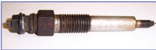
Figure 24 showing a worn out glow plug
