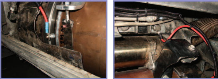
Figure 13 & Figure 14 showing the glow plug wired up (left) and the earth connection to outlet can
