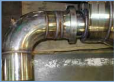
Figure 18 Boss for connection to service indicator
