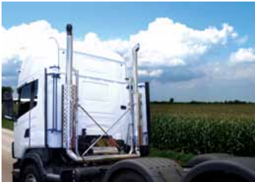
Twin stack conversion on Scania R620 Euro 4
