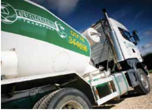
Single stack conversion on Scania R340 Euro 4
