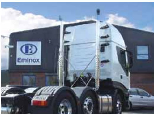
Twin tailpipe conversion on Iveco 480 Euro 5
