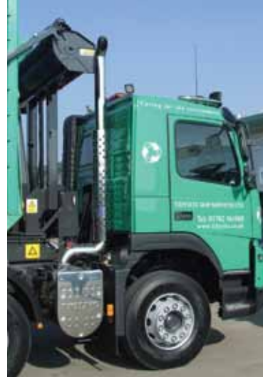
Single tailpipe conversion on Volvo FMX Euro 5
