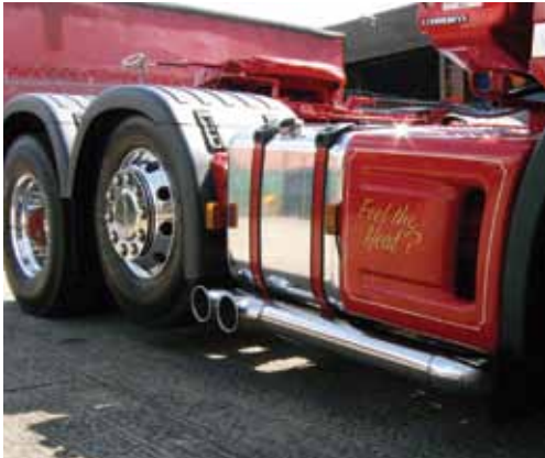
Side pipe conversion on Scania R580 Tractor Unit Euro 3
