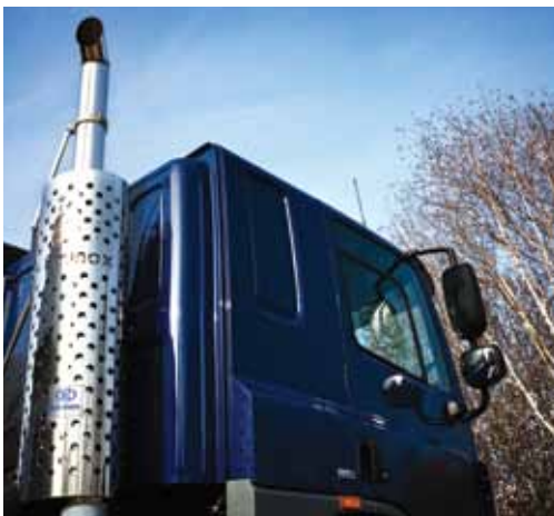
Single stack conversion on DAF 75.310 Euro 5
