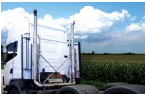
Twin stack conversion on Scania R620 Euro 4
