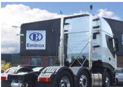
Twin tailpipe conversion on Iveco 480 Euro 5
