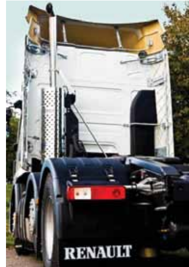
Single stack conversion on Renault Premium Euro 5
