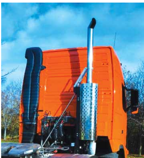
Single stack conversion on Volvo FH13 Euro 5
