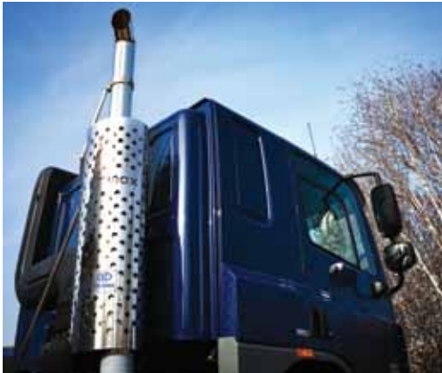
Single stack conversion on DAF 75.310 Euro 5
