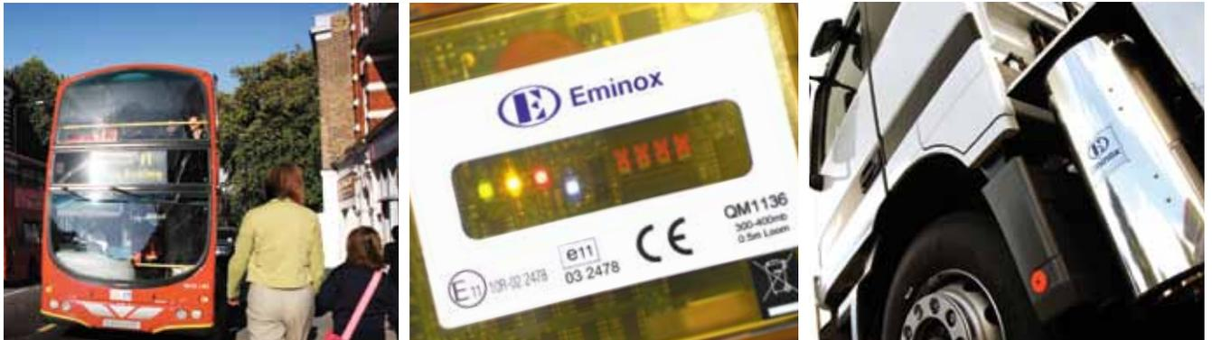
Eminox CRT® and SCRT® emissions systems rely on diesel particulate filters to maintain their particulate matter reducing capability. These filters need to be cleaned periodically to remove any build up of ash and particulate matter.
